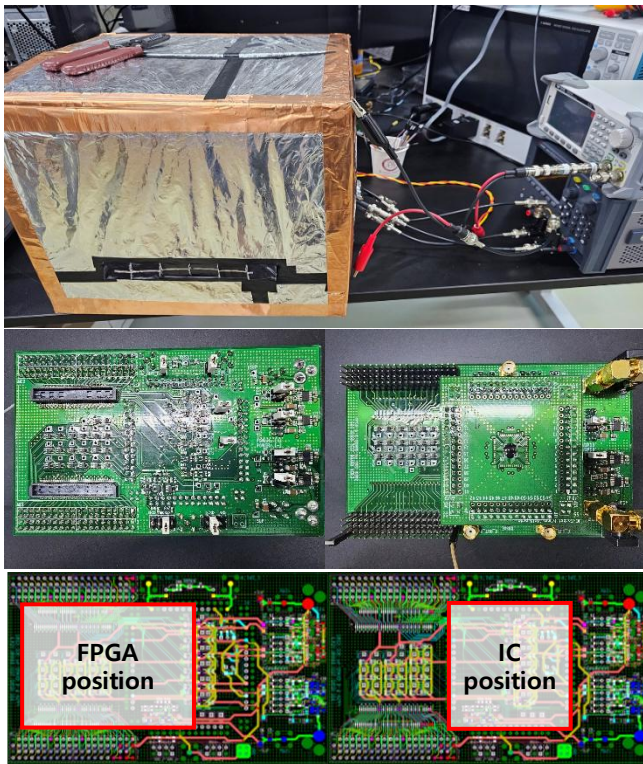
Fig. 7. The upper shows the overall test bench. A chipboard is placed inside the box to prevent interference from outer noise. Middle shows the PCB chip board. The left shows the FPGA connector part, and the right shows the IC connector part. Each part is on the opposite side of the one PCB. The bottom shows the PCB layout of the middle one.
