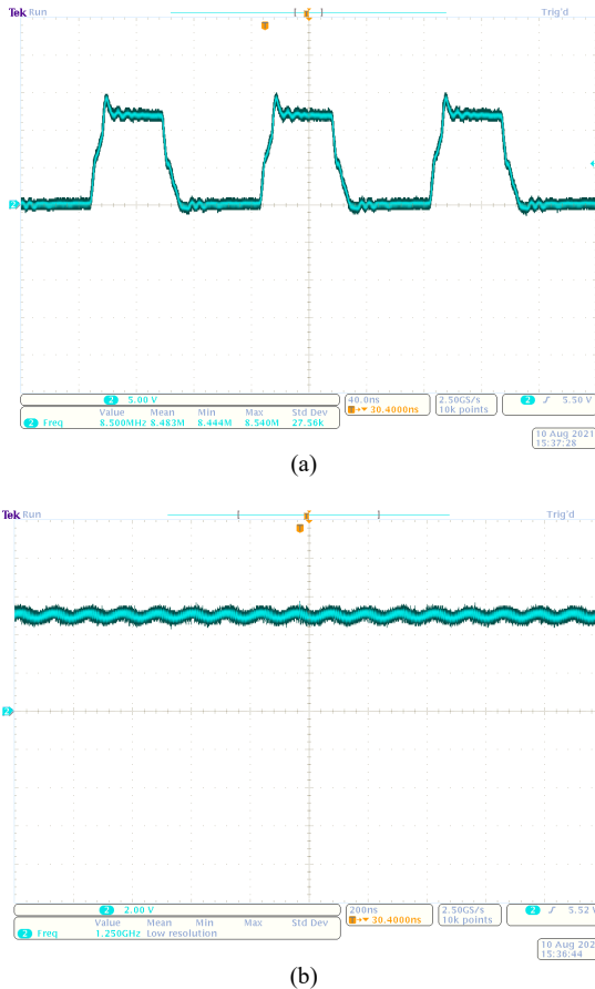
Fig 13. Chip test V_{SW} waveform and V_{OUT} waveform
