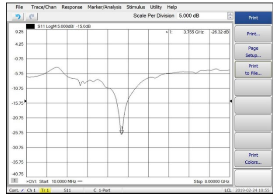
Fig. 8. Output matching performance of the proposed UWB pulse generator
