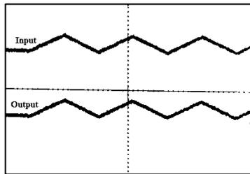
Fig. 12. Measured input and output voltages of the fabricated potentiostat chip.
