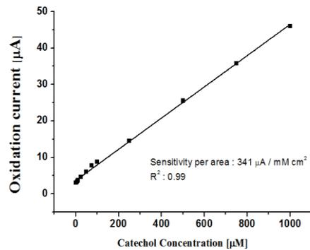
Fig. 4. Oxidation current measured at  $V_{\text{cell}}=0.58\text{V}$  in the cyclic voltammetry of Fig. 3 [1].
