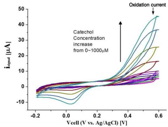
Fig. 3. Cyclic voltammetry curves with various catechol concentrations [1].
