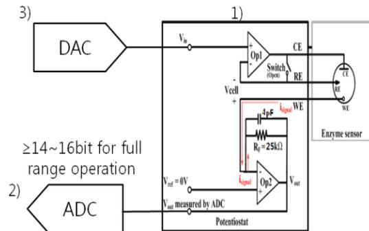
Fig. 1. A typical potentiostat driving an enzyme-based bio-sensor; 1) a potentiostat circuit; 2) an analog-to-digital converter; 3) a digital-to-analog converter.
