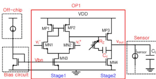
Fig. 6. A schematic diagram of the control amplifier (Op1 in Fig. 1).
