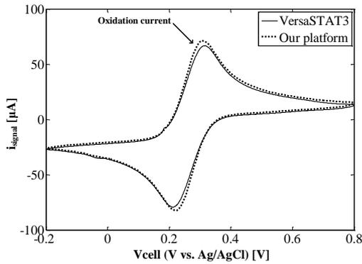
Fig. 5. A cyclic voltammetry curve of 5.0 mM  $K_3Fe(CN)_6$  in PBS buffer [1].
