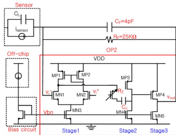
Fig. 8. A schematic diagram of the transimpedance amplifier (Op2, in Fig. 1).
