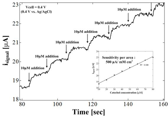
Fig. 2. Steady state current response (amperometry) of the laccase to successive 10µM increments of catechol in PBS [1]. The applied Vcell voltage is 0.4V vs. Ag/AgCl. Inset: i<sub>signal</sub> vs. catechol concentration.
