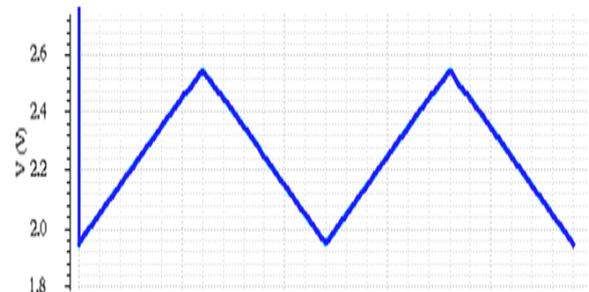
Fig. 7. A simulated output waveform of the designed Op1 in cyclic voltammetry.
